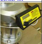
Tachometer with digital display to read shaft RPM
