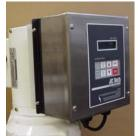
Tachometer with digital display to read shaft RPM
