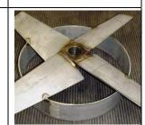
Stabilizer ring used to support long shafts
